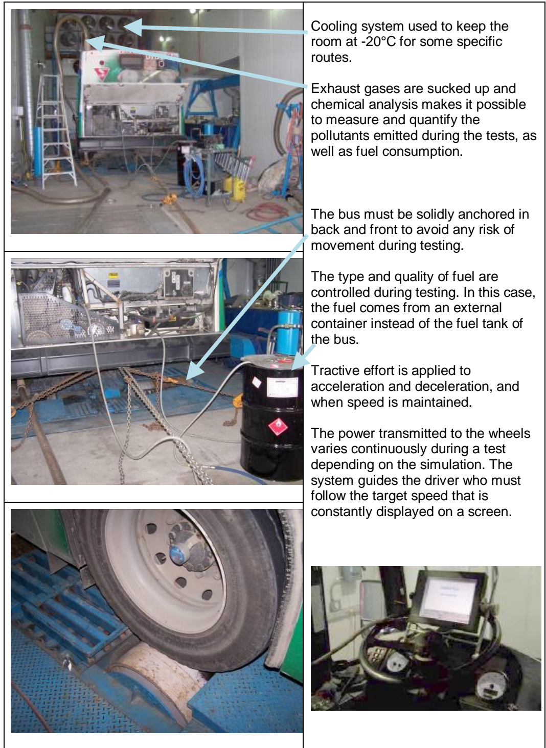
Figure 2-5 Tests at the Environment Canada laboratories
